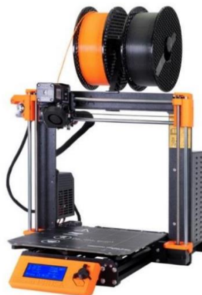
Slika 3.1. Original Prusa i3 MK3S 3D printer [6]
